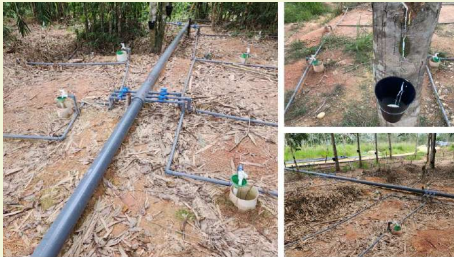
Figure 2: An illustration of a Typical ISL Mining of IAC RE Deposit in Perak
