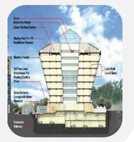
**Design features:** From the dome over its roof to its sunken garden and car park, every space within the Diamond Building is designed with functionality using stateof-the-art technology to optimise energy and water efficiency and indoor and outdoor environmental quality.
