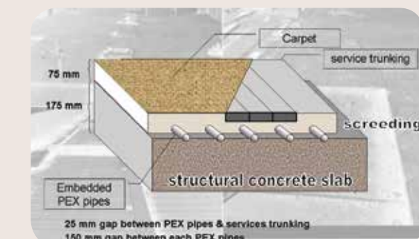
Close up view of the PEX pipes installation in Floor Slabs
